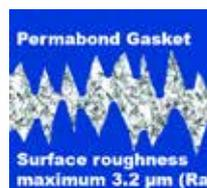
Not only do liquid gasketing adhesives give 100% contact between metal parts, but they also allow the engineer to cut down the amount of surface-finish machining, therefore reducing costs and increasing production rate.
