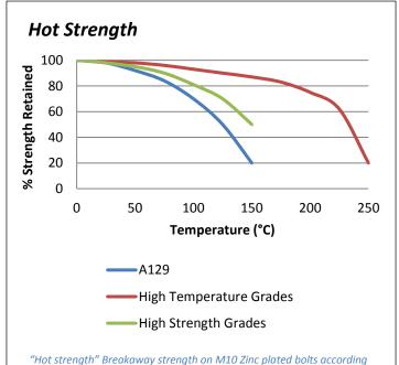
to ISO 10964. Cured at 23°C for 24 hours then conditioned for 30 minutes at testing temperature.
