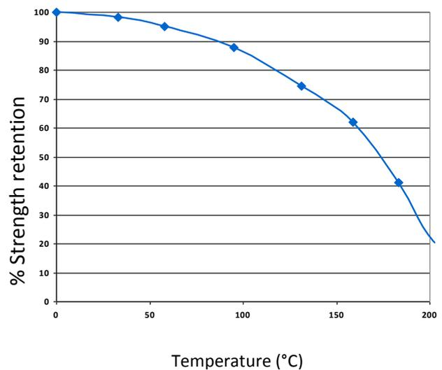
ES578 can withstand higher temperatures for brief periods (such as for paint baking and wave soldering processes) providing the joint is not unduly stressed. The minimum temperature the cured adhesive can be exposed to is -40°C (-40°F) depending on the materials being bonded.
