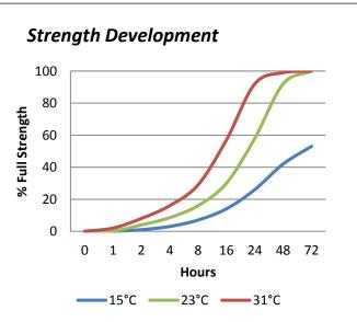
Graph shows typical strength development of bonded components. An increase of 8°C in temperature will halve the cure time. Lower temperatures will result in a slower cure time.
