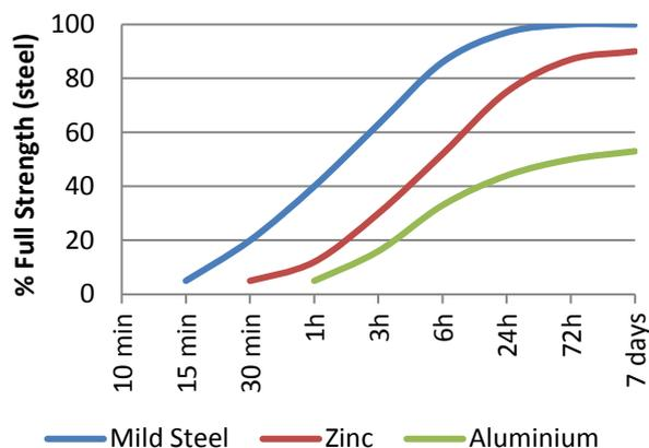
\*Cure times are typical at 23°C. Copper and its alloys will follow the faster cure while oxidised or passivated surfaces like stainless steel will tend towards the slower curve. Lower temperatures or large gaps will tend to extend the cure time. To reduce the cure time the use of Permabond A905, ASC10, or heat can be considered.
