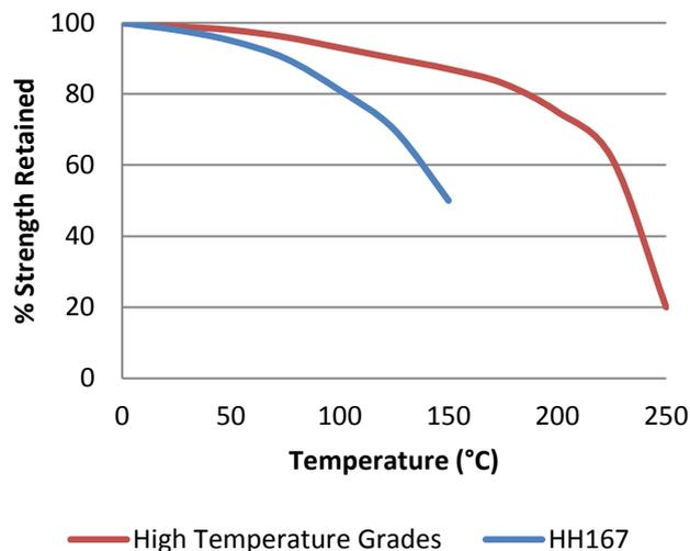
"Hot strength" Breakaway strength on M10 Zinc plated bolts according to ISO 10964. Cured at 23°C for 24 hours then conditioned for 30 minutes at testing temperature.
