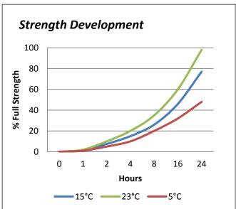
Graph shows typical strength development of bonded components. Increasing the curing temperature will result in a faster cure, colder conditions may slow cure slightly, but this is less marked than with most other epoxies.
