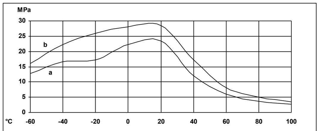
Roller peel test (ISO 4578) Cured 16 hours/40°C
