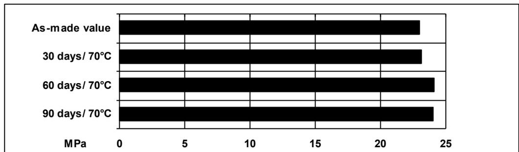
**Lap shear strength versus tropical weathering**
