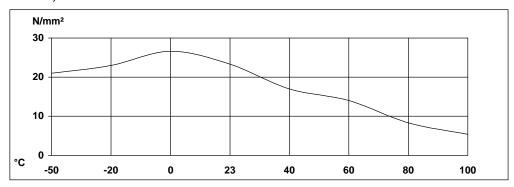
Roller peel test (ISO 4578) at 23°C 6 N/mm
