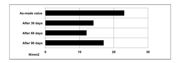
Shear modulus (DIN 53345)
