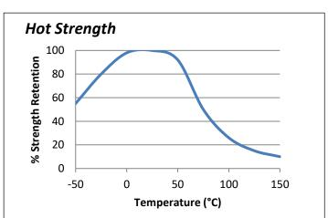
"Hot strength" shear strength tests performed on mild steel. 24hr cure at room temperature and conditioned to pull temperature for 30 minutes before testing.
