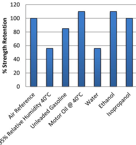
Specimens were immersed for 1000 hours at 22°C (unless otherwise stated).
