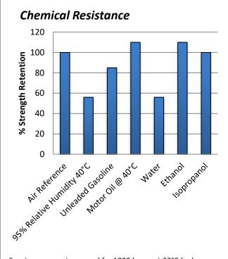
Specimens were immersed for 1000 hours at 22°C (unless otherwise stated).
